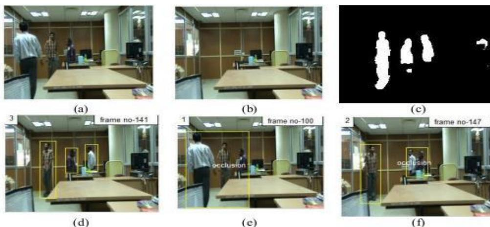
Fig. Object tracking process (a) Video Sequences, (b) Background Model, (c) Background Subtraction, (d) Multiple Object Tracking with Bounding Box, (e) & (f) Occlusion Detection
