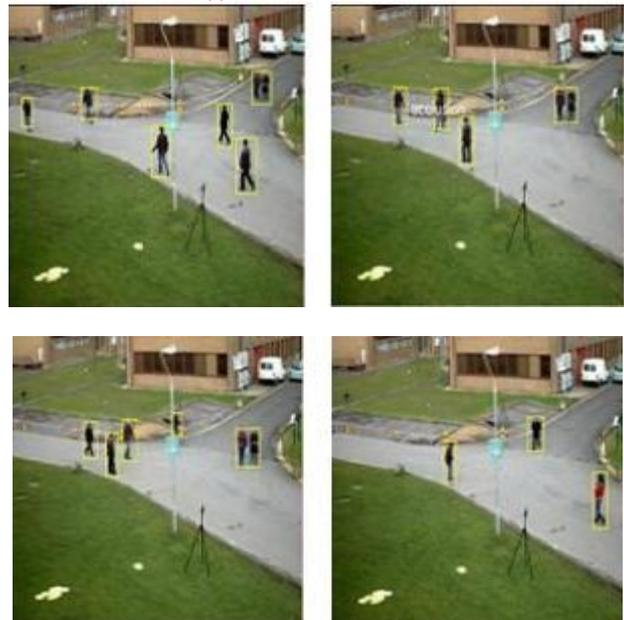
(b) Proposed background subtraction &amp; shadow Removal
