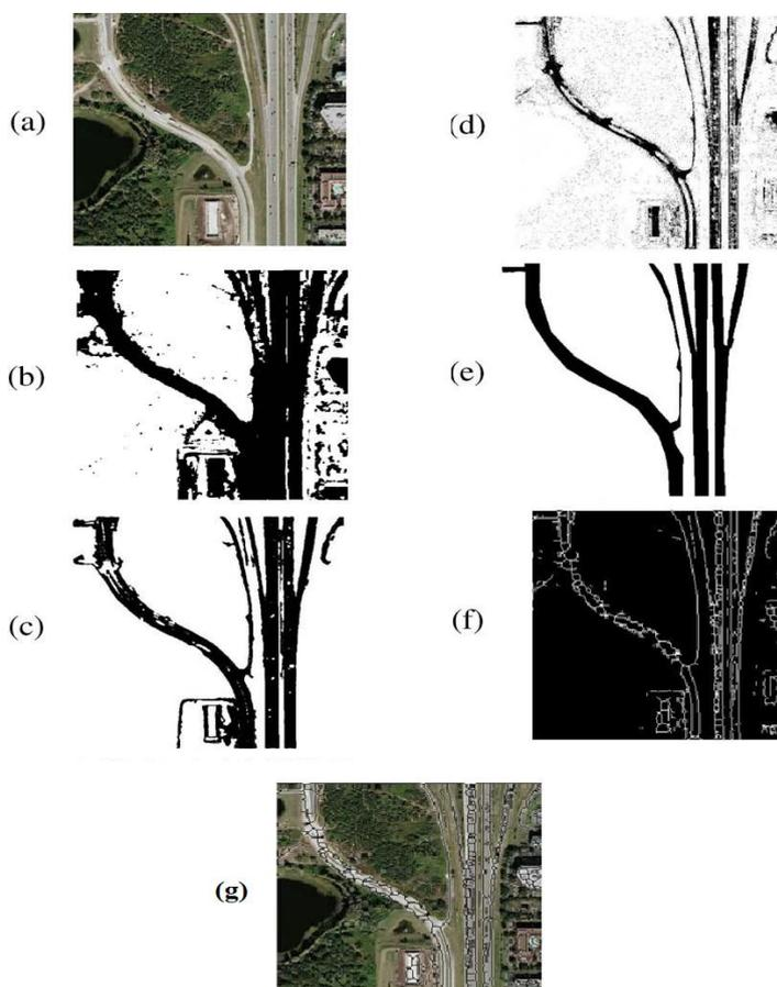
Figure3. (a) Four satellite images of size  $(512 \times 512)$  from a suburban area of a developed region. (b) Results from FeatureObjex [4]. (c) Results of the method proposed in [2]. (d) Results of the method proposed in [3]. (e) Hand-drawn (manual) road map (f) Results of method proposed in [5]. (g). Result of our proposed approach.
