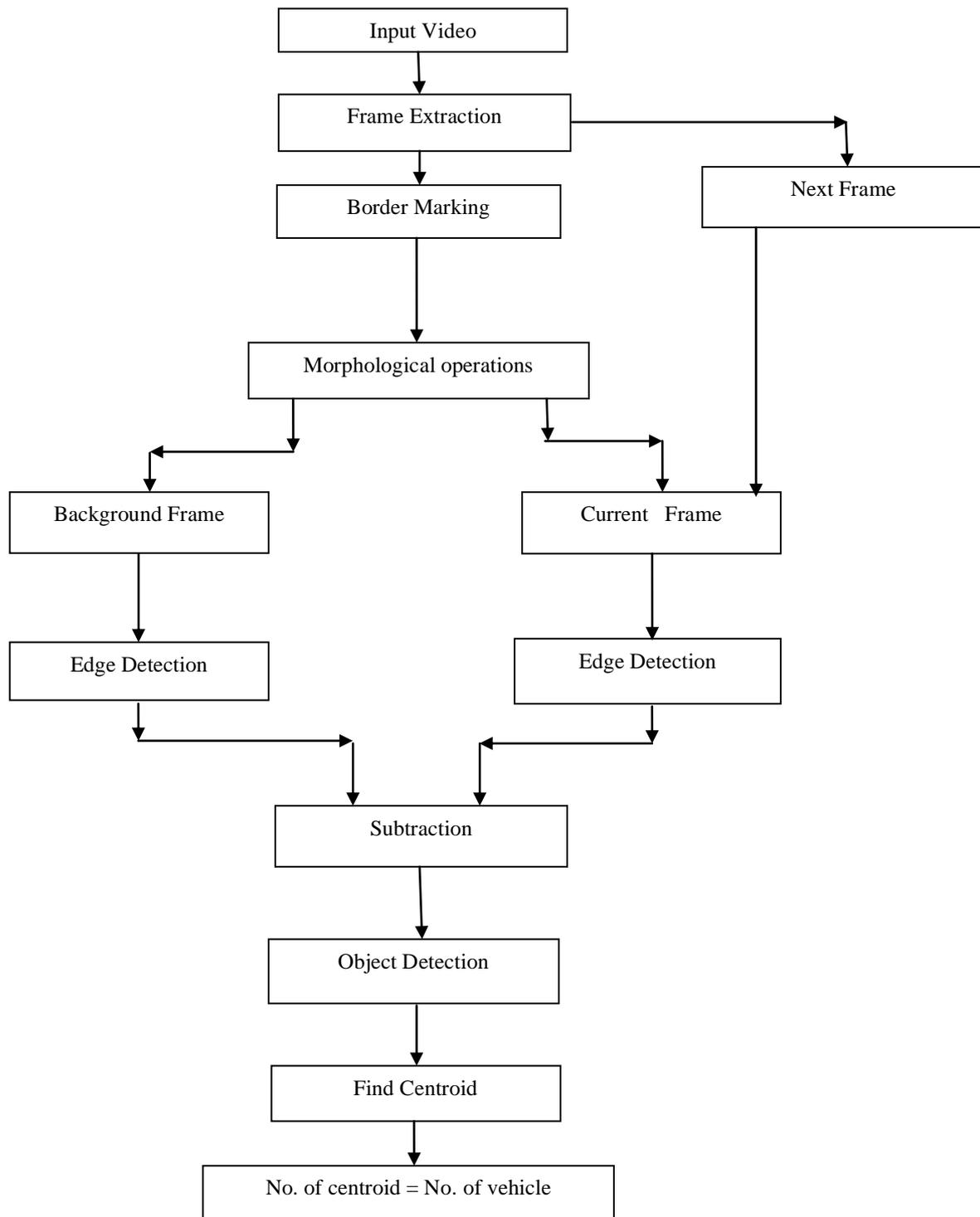
Figure.3.1: Flowchart for vehicle counting
