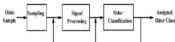
Fig. 2. Typical block diagram of the e-noses.
