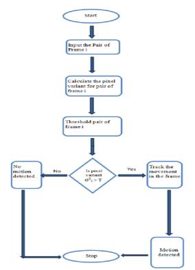
Fig. 3 Flowchart of motion detection method
