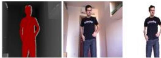
Fig. 2. Background removal. Depth image (left), color image (middle), extracted user image (right)
