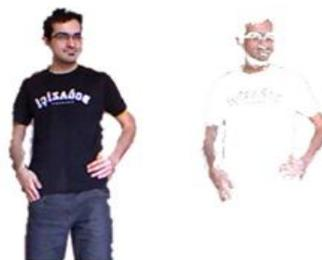
Fig. 3. Skin colour segmentation. User image (left), segmented image(right)
