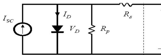
Fig. 2 Typical circuit of PV solar cell
