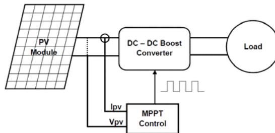
Fig. 1 Typical diagram of MPPT in a PV System
