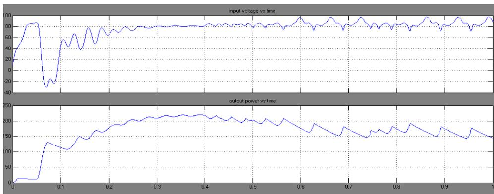
Fig.18 Input voltage and output power of incremental conductance using sepic converter.
