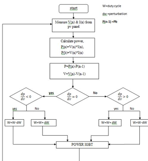
Fig. 3 Flow Chart of the P&O Method.
