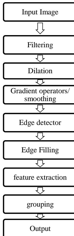
Fig. 2.1 Example of a typical image segmentation algorithm
