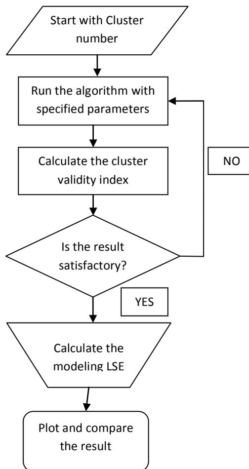
Fig. 3.1 Fuzzy C-Means clustering algorithm Procedure [11]
